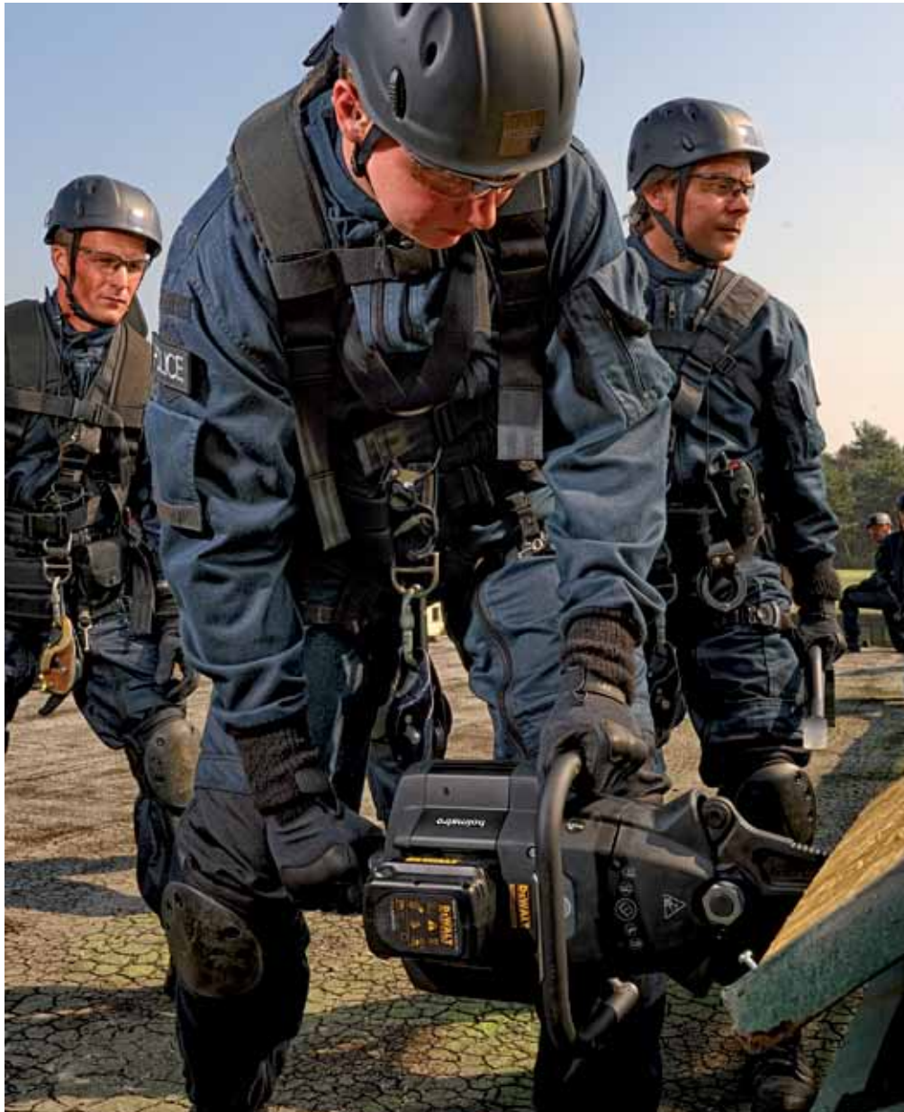
Spreading open a roof hatch and cutting the barred window (see page 8) with a Holmatro battery-operated combi tool.
