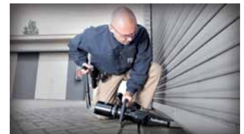
Tool and pump in one offering ultimate mobility (HPW 4624 ST).
